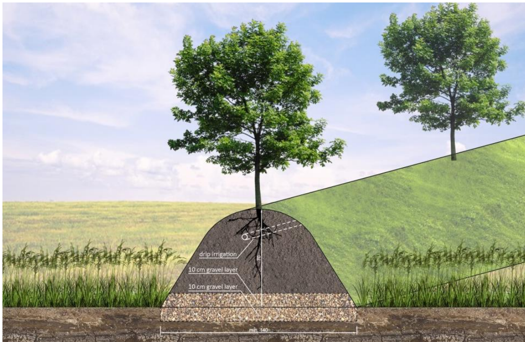
Figure 2.24 Dibbling process will be done on high ridge (around 70 cm high from soil surface level)
