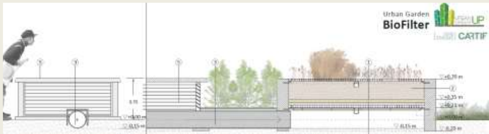
Figure 8. CARTIF. URBAN GreenUP Project. Biofilter cross section
