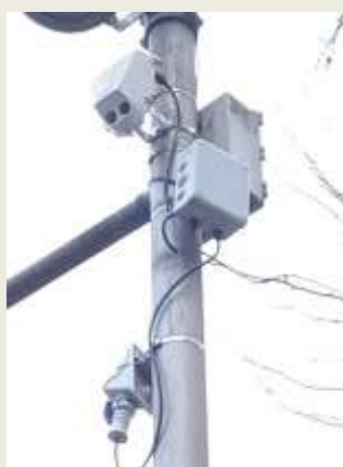
Equipment and methodology: Vivacity traffic sensor:
