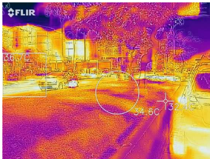
Figure 6.2: San Juan Corridor. After the green corridor. Decreases in radiant heat between 6°C and 8°C are shown at noon.
