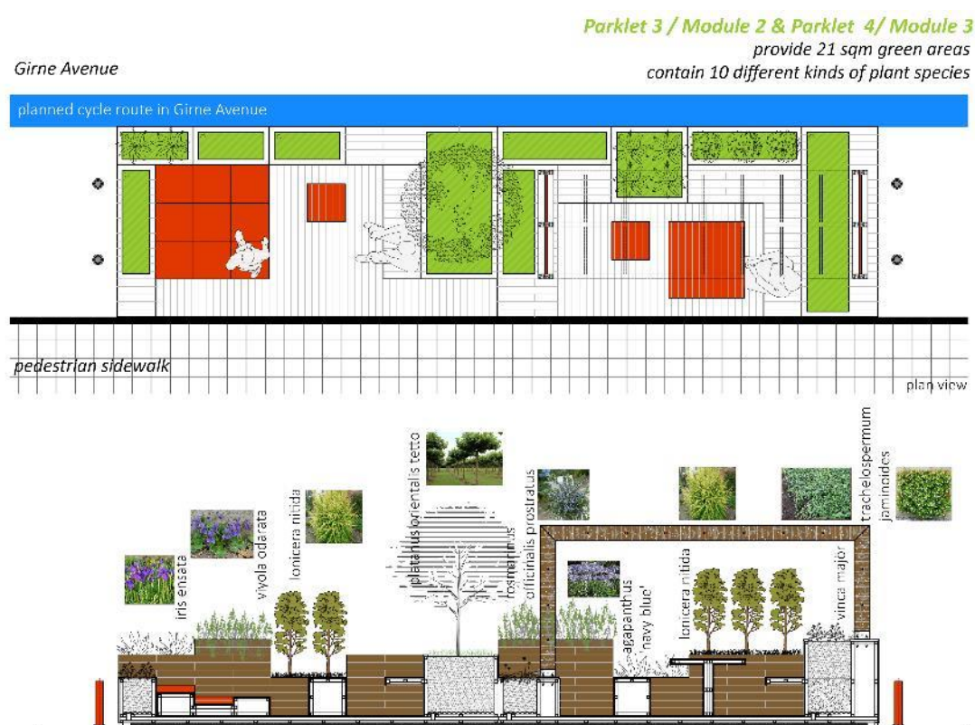
Figure 2-7: Technical Drawing of Parklet modules #3 & #4
