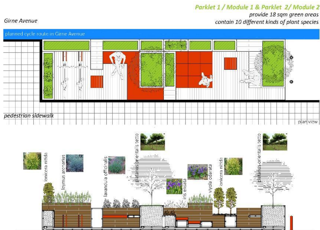
Figure 2-6: Technical Drawing of Parklet modules #1 & #2
