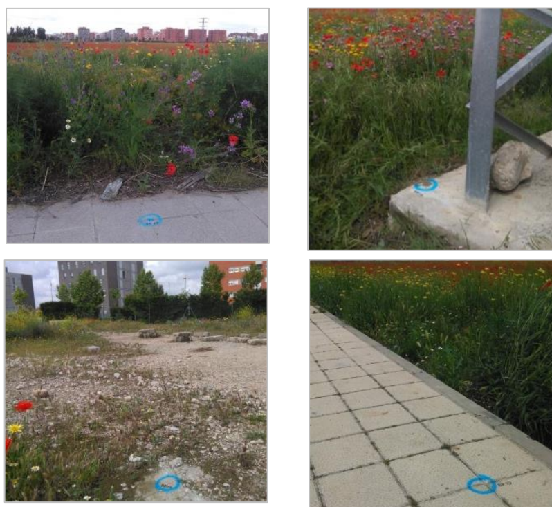
Figure 4.44: Stakeout bases used for the topography study (Source: Duero River Basin Authority).
