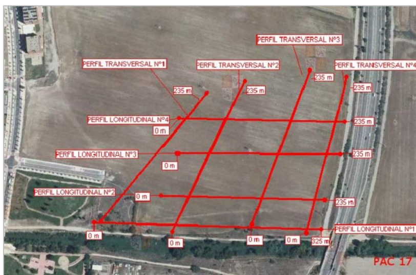
Figure 4.48: Location of the wire lines used to carry out the Electrical Tomography (Source: Google/Duero River Basin Authority elaboration).
