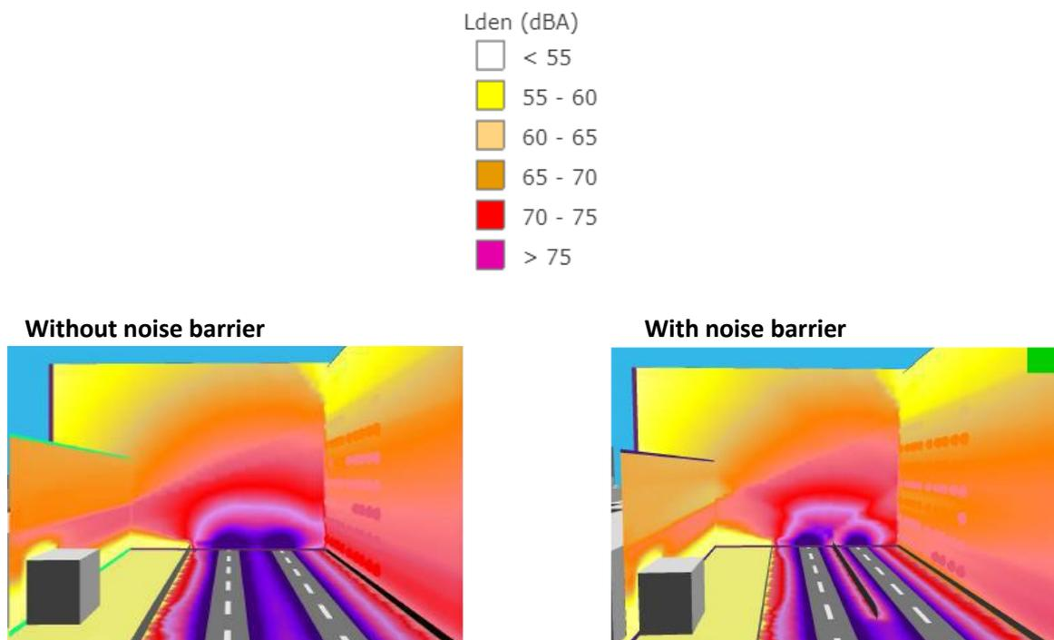
Figure 17. Simulation of absorbed noise with the Green noise barriers.
