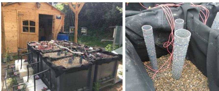
Figure 3.1: Electro-wetland prototype built in LEITAT headquarters (Barcelona)
