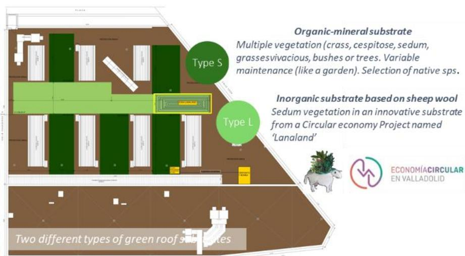
Figure 26: Two different types of green roof substrates (Vac28).
