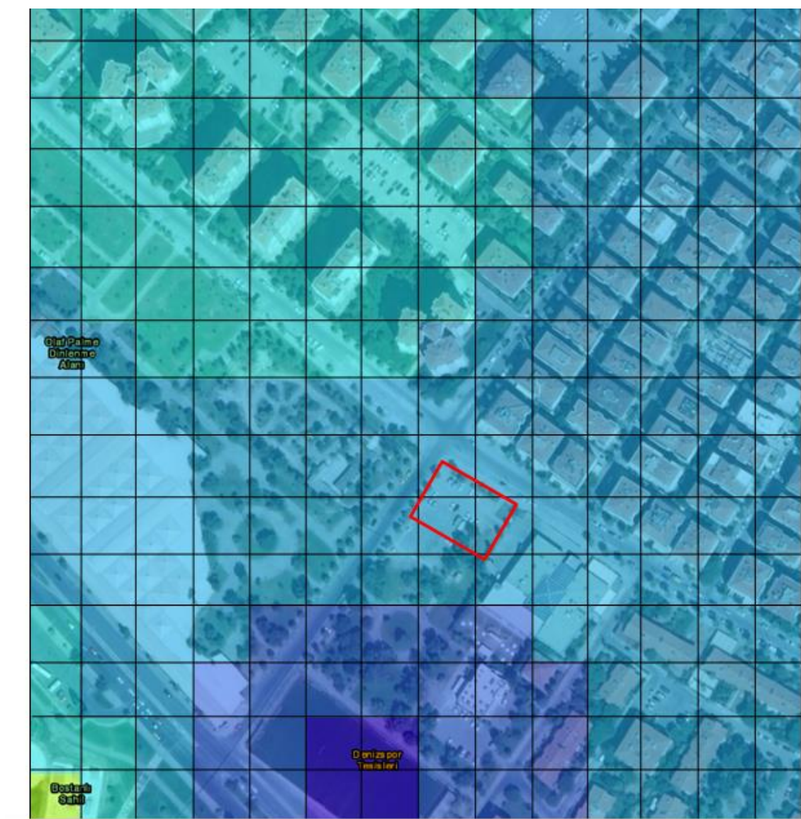
Figure 2-7 Landsat-8 LST 30 m grid overlapped with high resolution image – Study area 2
