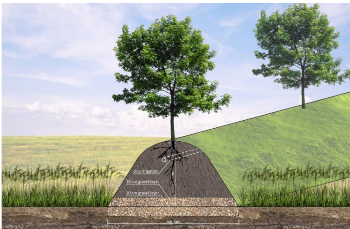
Figure 3-18: Schematic view of high ridge seeding system
