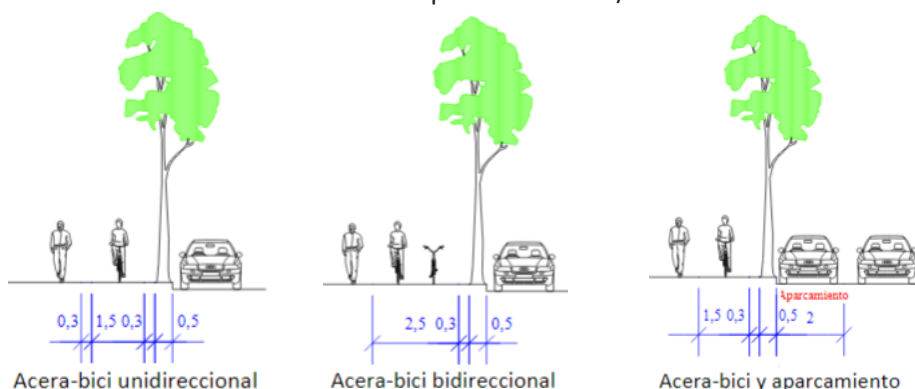
Figure 2.9: Segregated cycle-sidewalk section (Source: revision PGOU 2017)
