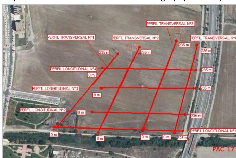
Figure 4.48: Location of the wire lines used to carry out the Electrical Tomography
