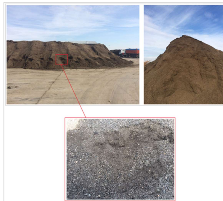
Figure 28 Smart soil made from sludge and agro-food waste
