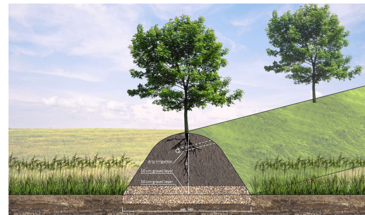
Figure 56 Layers to prevent soil from salty ground water
